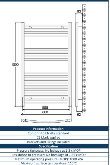
Resistance against corrosion: No corrosion after 100 h humidity
