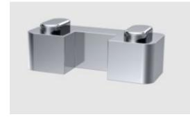
35362101 is a Support Foot and is an optional extra for use with Wet Room screens. It is designed to ensure extra support around the glass panel. (Please note you cannot screw through this part into a tanked floor as it will breach the integrity of the tanking).
