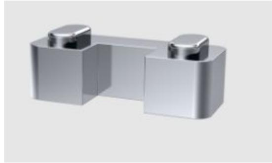
35362101 is a Support Foot and is an optional extra for use with Wet Room screens. It is designed to ensure extra support around the glass panel. (Please note you cannot screw through this part into a tanked floor as it will breach the integrity of the tanking).
